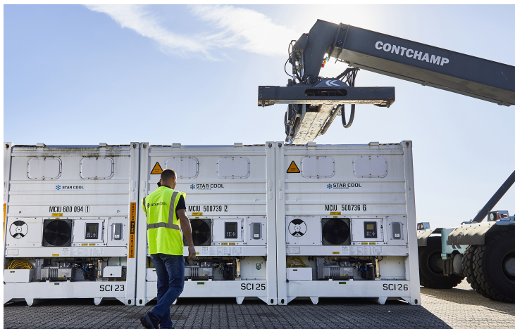
Figure 4.1: MCI Starcool reefers. The cooling fan, compressor, user display, and electronics box are clearly visible on each reefer.
